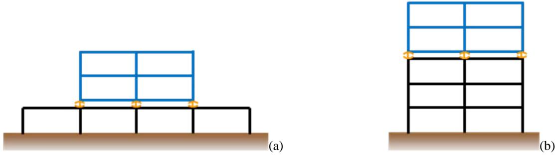
Figure 5 – Hybrid model configurations, blue indicates the physical specimen, black indicates the substructure: (a) Model A (b) Model B
