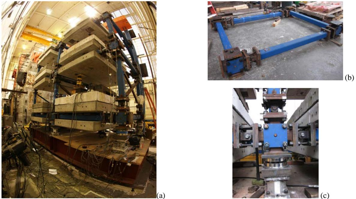
Figure 3 – (a) Isolated frame superstructure installed on the shake table (b,c) REPEAT frame components
