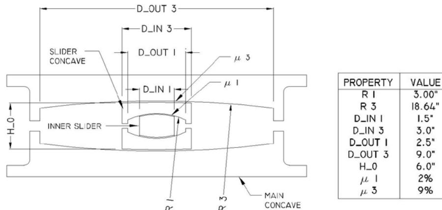
Figure 4 – Triple friction pendulum cross section and properties
