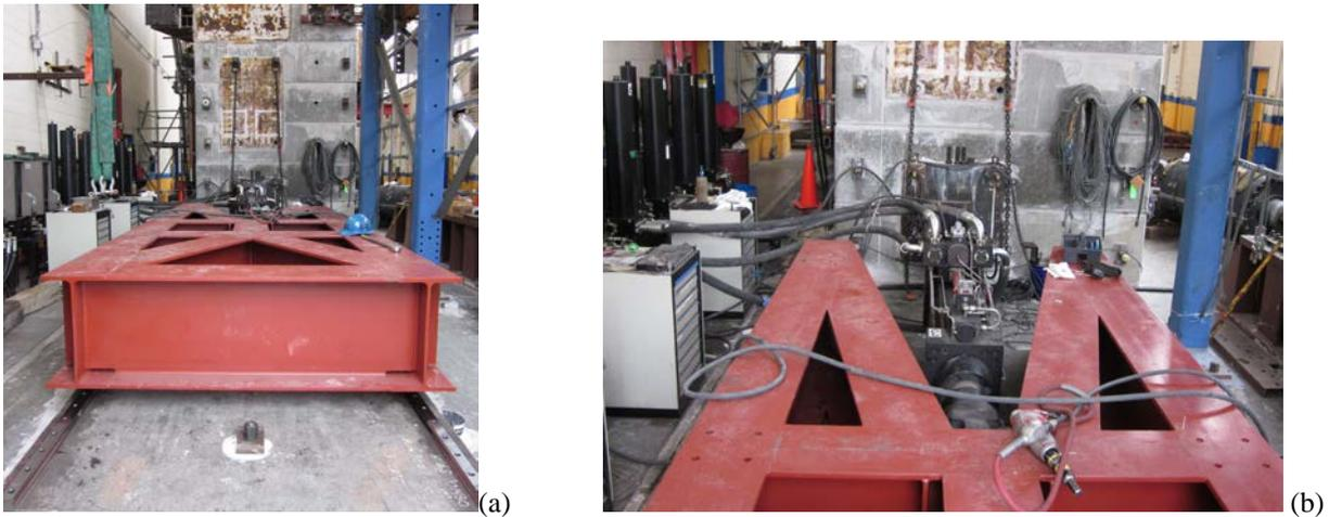
Figure 1 – Unidirectional shake table
