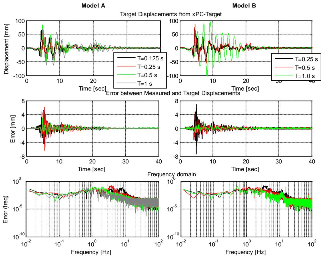
Figure 6 – Numerical substructure top displacement, error between target and measured displacements to the physical superstructure and FFT of the error for the various substructure configurations
