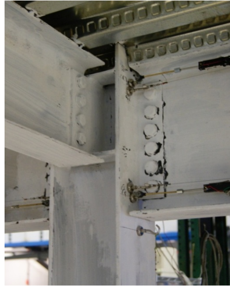
(c) Shear-Tab Conn. "C" [+0.015 rad.], HS02-100%
