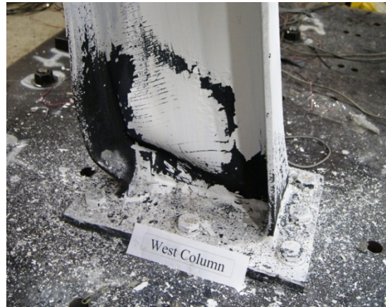
(f) West Column [0.146 rad.]; Test ID: HS01-200%
