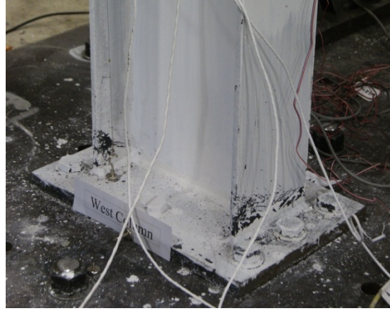
(b) West Column [0.003 rad.]; Test ID: HS01-100%
