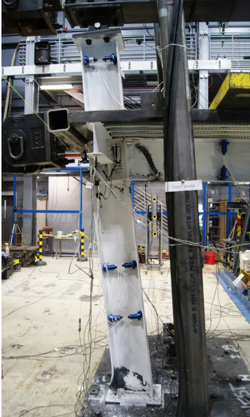
(a) North view of deformed east column
