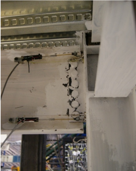
(b) Shear-Tab Conn. "B" [-0.006 rad.], HS02-25%
