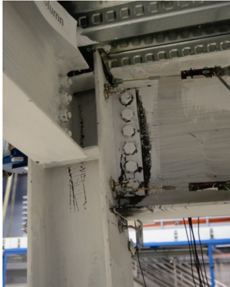
(e) Shear-Tab Conn. "A" [-0.069 rad.], HS02-200%
