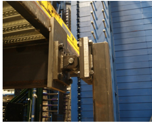
(b) Clevis between test specimens and vertical link member
