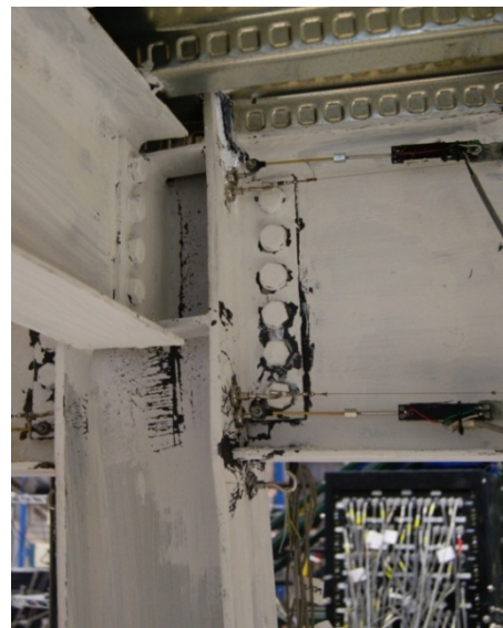
(e) Shear-Tab Conn. "C" [-0.048 rad.], HS02-200%
