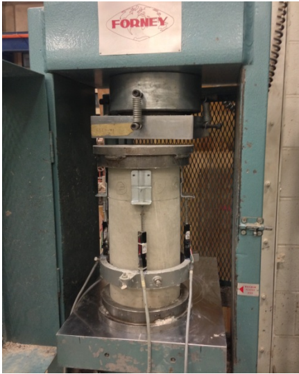
(a) Standard cylinder test
