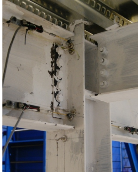
(c) Shear-Tab Conn. "B" [+0.014 rad.], HS02-100%
