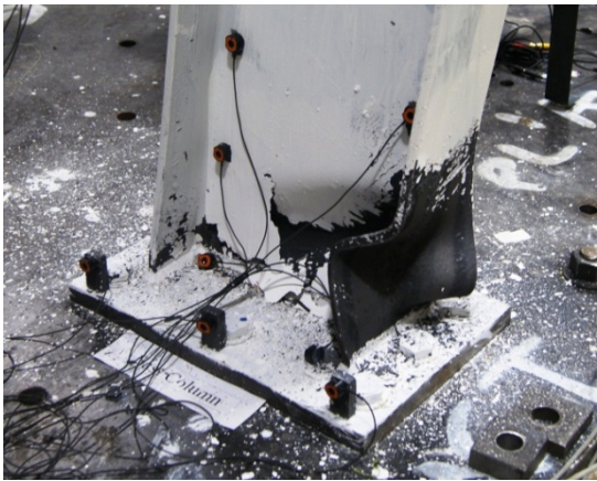
(e) East Column [0.165 rad.]; Test ID: HS01-200%
