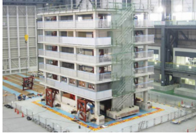
Figure 2-6 Full-scale six-story reinforced concrete structure tested at E-Defense (Kim et al. , 2012)
