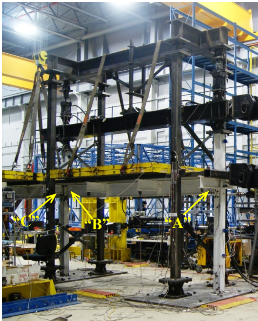
(a) Location of shear-tab connections
