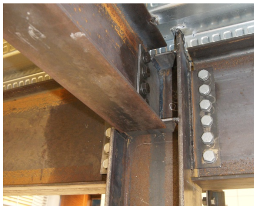
(c) West joint of gravity frame test specimen
