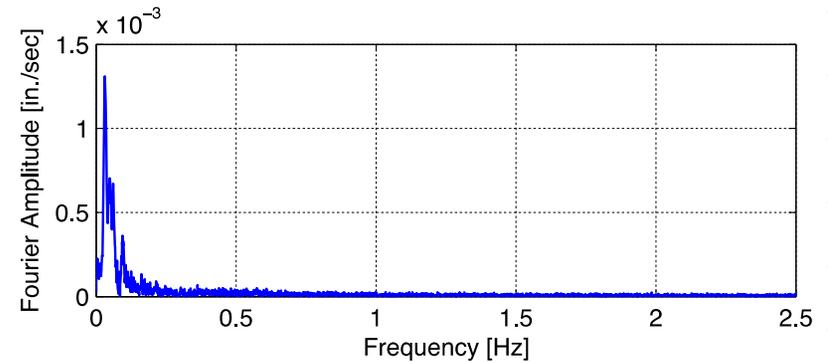
The only frequencies that were picked up in the Fourier amplitude spectra were the frequencies of the structural response in the two directions (0.062 Hz in the global X-direction and 0.031 Hz in the global Y-direction)
